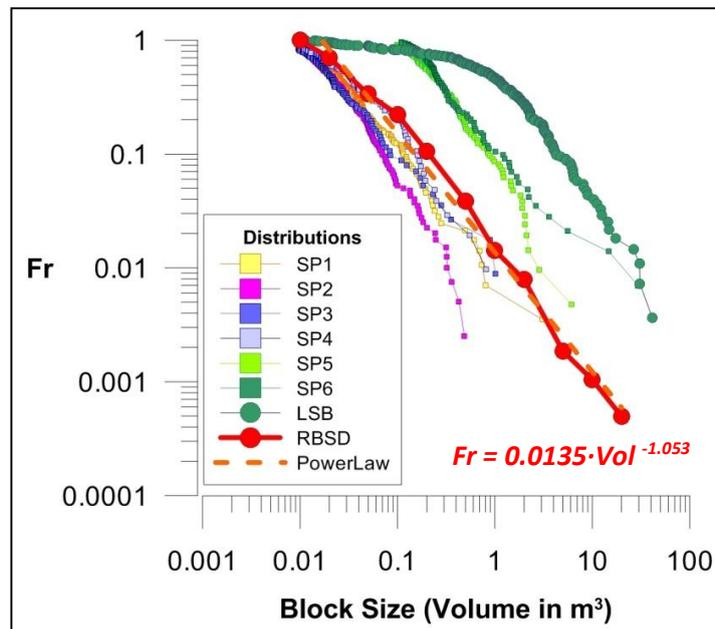
Fig.3: Block size distribution obtained from the 6 sample plots: SP1-6; from the large scattered blocks measured: LSB, the obtained Rockfall Block Size Distribution: RBSD, and the fitted power law (the four largest scattered blocks excluded).
