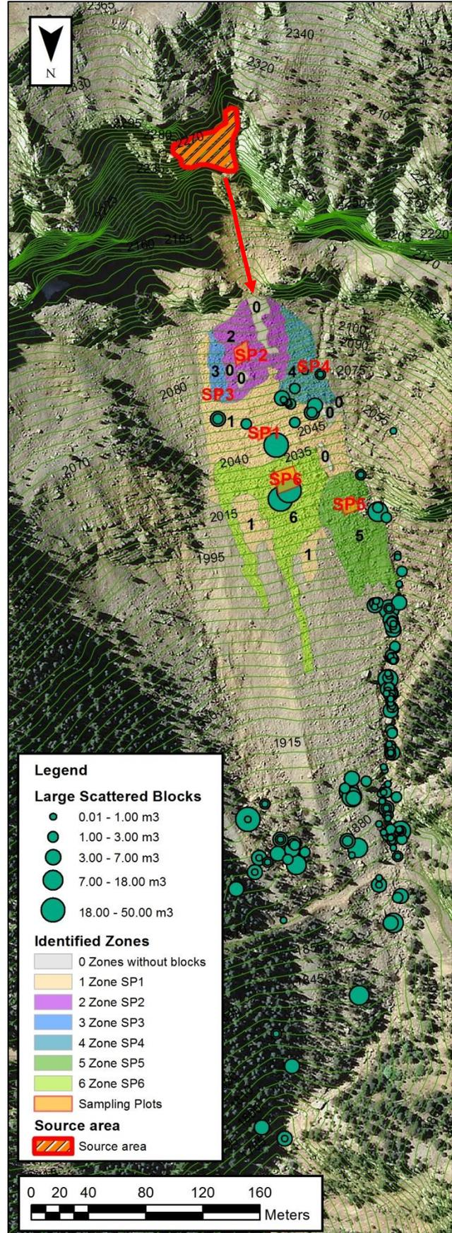
Fig. 2: Orthophoto map showing the location of the six homogeneous zones of the YDC, sampling plots, the large scattered blocks, and the source area.
