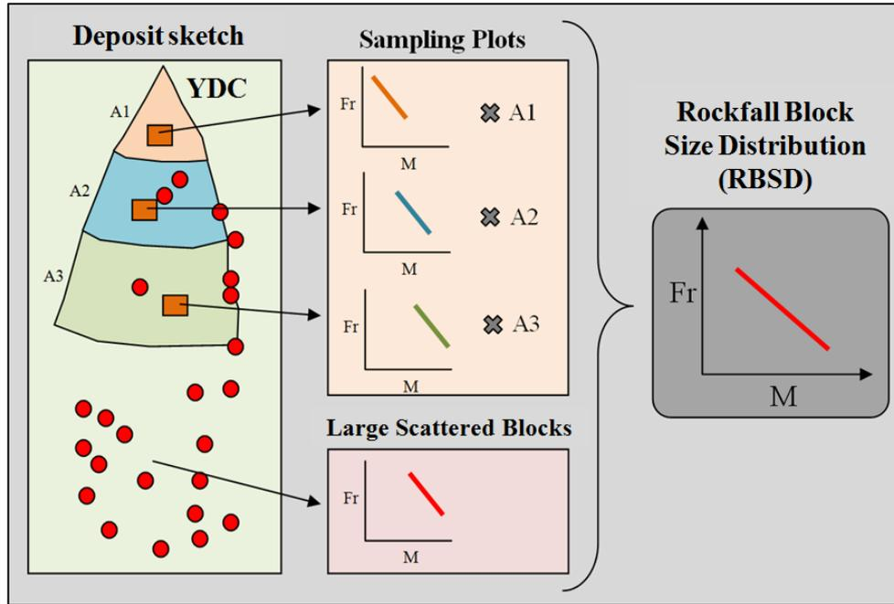
Fig. 1: Methodology followed to prepare the RBSD. The scheme shows the YDC, the sampling plots for each homogeneous zone A1 to A3, and the large scattered blocks. The plots display the block size distribution where "Fr" is the cumulative relative frequency for each block size bin "M".
